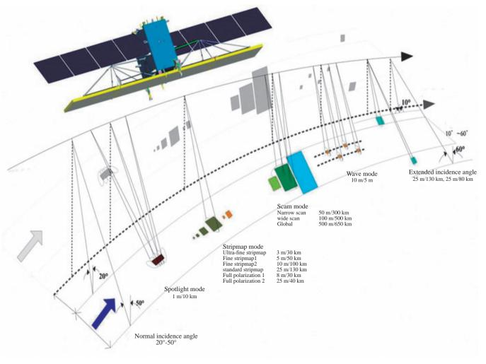
Figure 3 GF-3 satellite imaging modes
