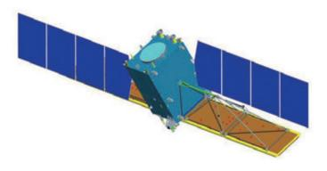
Figure 2 Attitude of GF-3 with right sidelook in orbit
