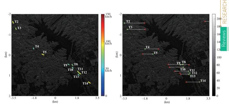
Figure 11 GF-3 satellite moving target detection and reposition results
