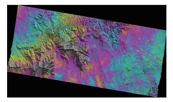
Figure 10 GF-3 satellite differential interference phase diagram in Songshan area (10 m grid)
